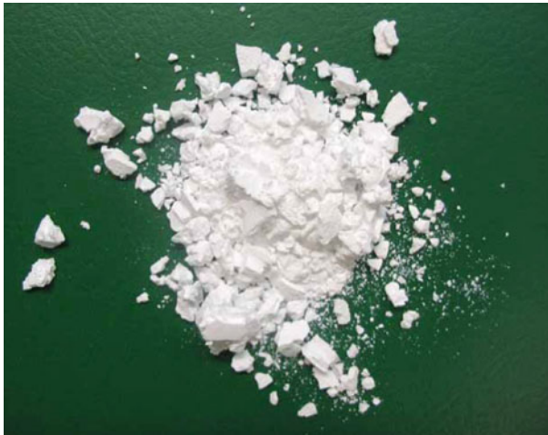
Fig. 7 Recycled materials obtained from steel converter slag used in CO 2 fixation processes
